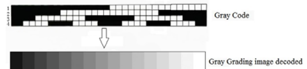
FIGURE IV. GRAY CODE IMAGE DECODE TO GRAY GRADING IMAGE.
