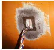
Fig.2 Welding position diagram of strain gauge.
