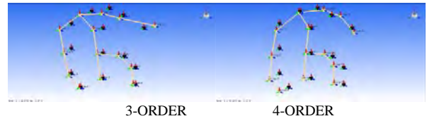
FIGURE IX. THE FIRST 4-ORDER MODAL VIBRATION RESULTS OF POSTURE 1
