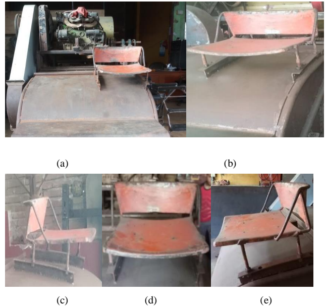
Fig.2. Design of Combine Harvester Machine Seating (a, b) The overall seating picture (c) Seat drawing from the left side (d) Image of the front (e) Right side image
