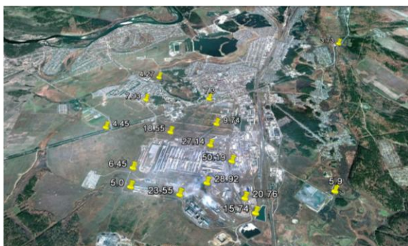
Fig. 2. Representation of the field of SO 4 emissions into atmosphere close to Heat-and-Power Plant (Shelekhov town, Irkutsk Region).
