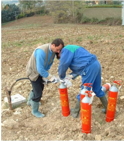
Fig. 7 Field figure of gas leakage simulation
