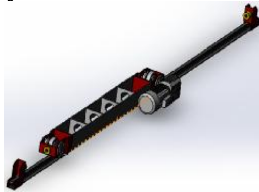
Fig. 2 conveying guide system
