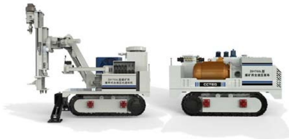
Figure 3: the floor anchor drill rig general view
