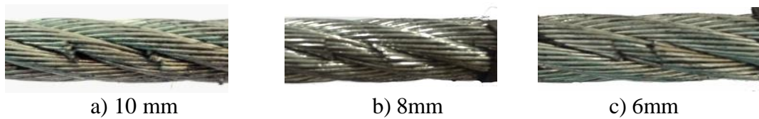
Fig.3 Section of broken wires faults
