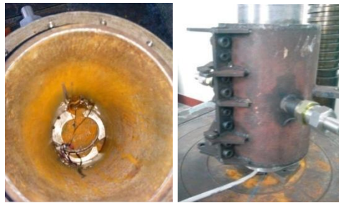
Fig. 9. The distribution of strain gauges
