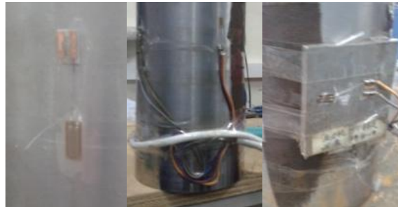
Fig. 7. The distribution of strain gauges
