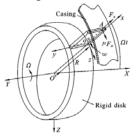
Figure 2. Dynamic modal of hub-plate system with rubbing
