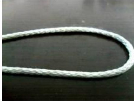
Fig .2 PEEK/LQ 3D-braided prepreg
