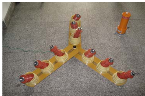
Fig.6 The fixed arrester
