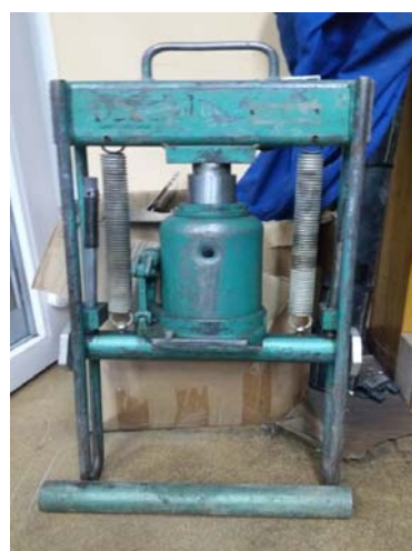
FIGURE II. SQUEEZE – OFF TOOL USED FOR SHUTTING OFF THE POLYETHYLENE PIPES OF 63 – 160 MM DIAMETER
