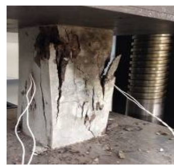
Fig.4. The elastic modulus test of full lightweight aggregate concrete
