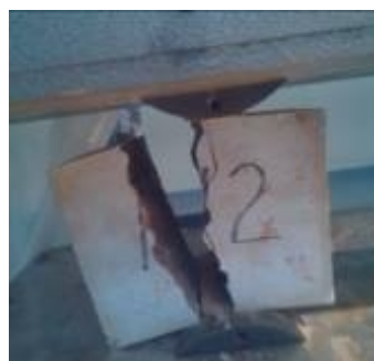
Fig.3. The cleavage strength test of full lightweight aggregate concrete
