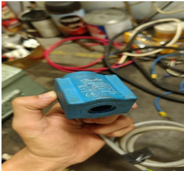
Fig. 5. Damaged Solenoid Valve
