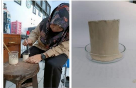
Fig. 1. The coating process on stainless steel pipes as a prototype.
