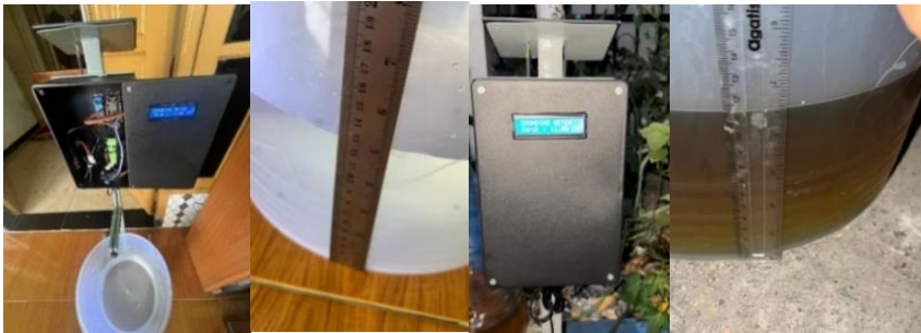
Fig. 10. JSN-SR04T Sensor Testing on Water and Diesel B30. Source: Personal Documentation
