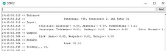
Fig. 15. Fuzzy Calculation from Arduino
