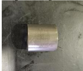
Fig. 5. Less hardness, a condition where there are dark straight lines or dots.
