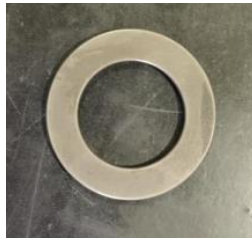
Fig. 2. Grinding Burn, a condition in which there are soft spots and light and dark areas that contrast with the background of the material.
