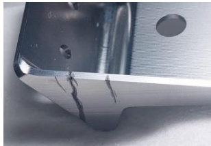
Fig. 6. Cracks, where there are dark serrated lines and sometimes burn conditions.
