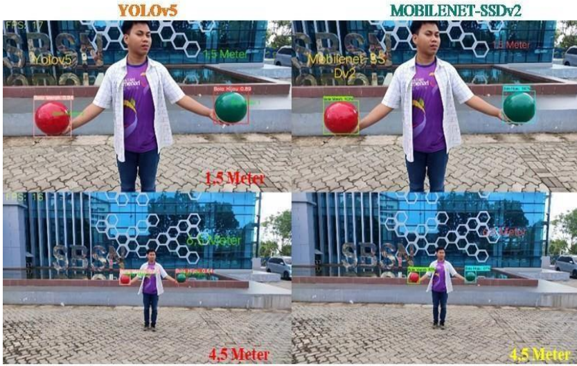
Fig. 5. Object detection distance of YOLOv5 and MOBILENET-SSDv2 algorithms.
