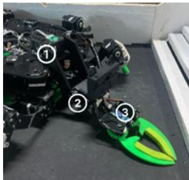
Fig. 11. Position of the servos on the gripper
