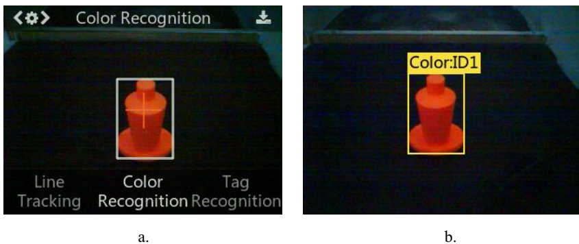
Fig. 9. (a) Learning process on color recognition algorithm, (b) Learning result on color recognition algorithm
