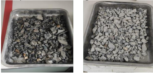
Fig. 4. Aggregate water absorption test (left is saturated surface dry state, right is after drying).
