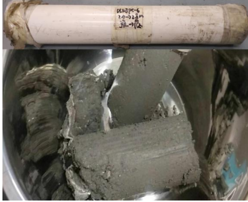
Fig. 1. Coring samples of the SCS
