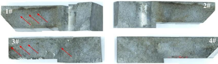
Fig. 2. Macroscopic morphology of fracture surface of 1#-4#.
