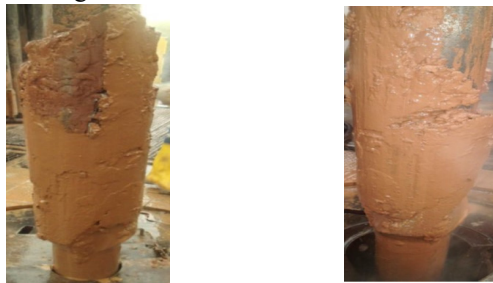
Fig. 2. Mud package of drilling tools at the drilling site of Oilfield A.
