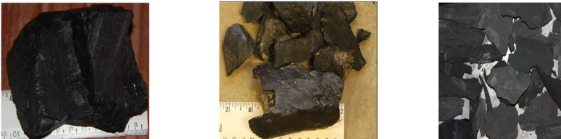
Fig. 1. Block falling during drilling process.
