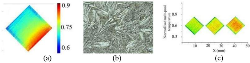
**Fig. 5.** (a) The melt-pool temperature profile [22], (b) optical micrograph showing the grain size distribution, and (c) the melt-pool temperature measure of 3 parts printed with 30, 60, and 90-microns layer thickness [9].
