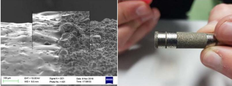
**Fig. 4.** SEM and optical images of an AM part showing the surface roughness before and after laser polishing [10]
