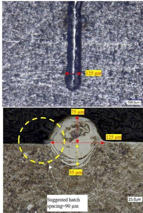
**Fig. 3.** The procedure used for calculating the hatch spacing in a L-PBF process [20]
