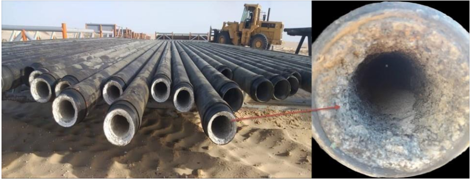
Fig. 1. Scale formation in A71 well production tubing.
