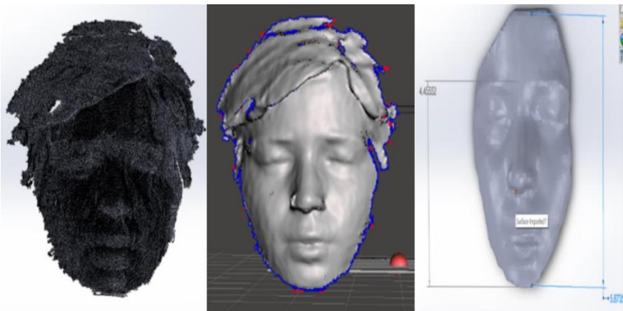
Fig. 3. Facial feature acquisition: (a) raw scan with noise (b) close whole mesh body (c) 3D adapted mesh model that has been intricately modified through computational methods.
