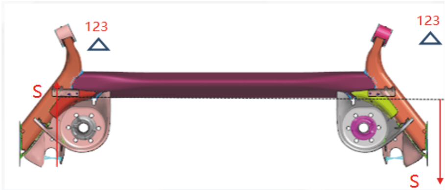
Fig. 10. Torsional fatigue simulation model
