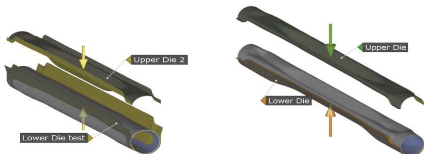
Fig.5. Finite element simulation model of preforming and hot metal gas forming
