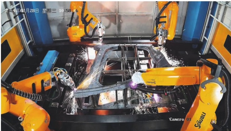
Fig. 9 Four robots working together for body door ring cutting
