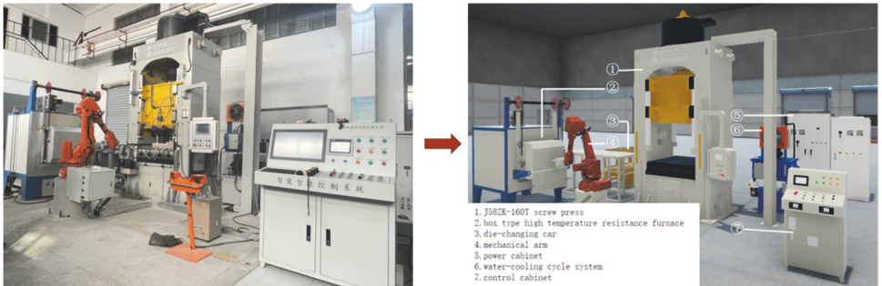
Fig.2 Physical and virtual geometric model of 1600kN electric servo screw press
