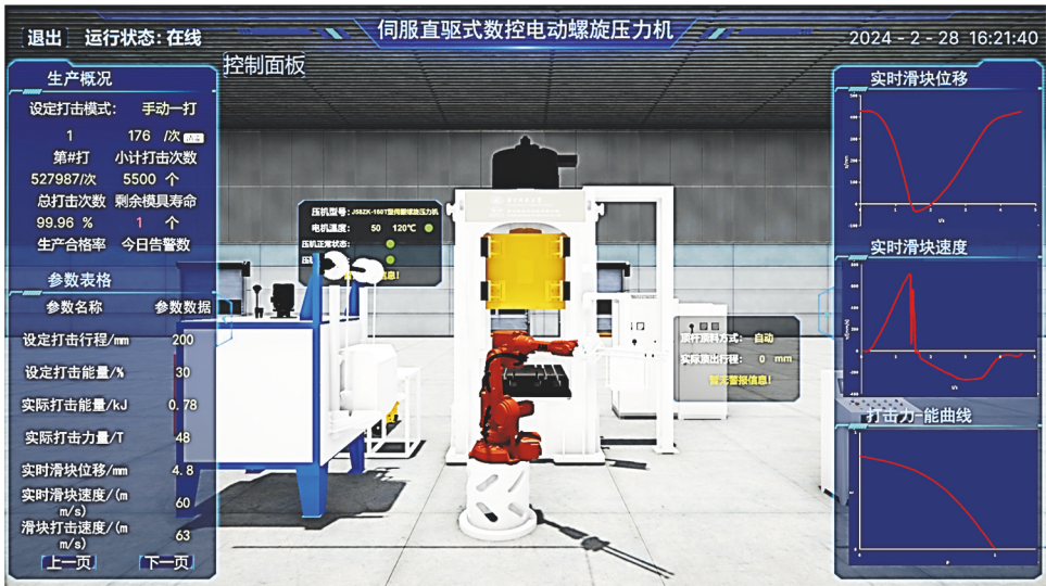
Fig.3 Three-dimensional visual monitoring interface of 1600kN electric servo screw press
