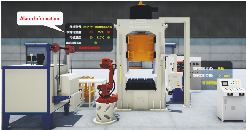
Fig.4 Visual alarm interface of 1600KN electric servo screw press
