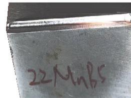
Fig. 4 photos of the lower module and the tested steel plate welded on the module surface
