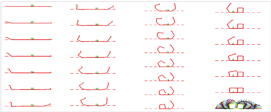
Figure 12 Optimized roll forming process flow diagram
