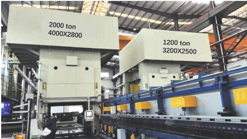
Fig. 7 Double press-roller-hearth furnace flexible production line in actual operation
