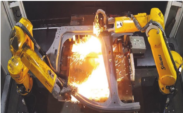
Fig. 6 Twin-robot, two-head cutting system (door ring part cutting)
