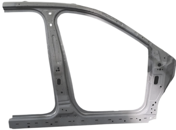
Fig. 9 Actual picture of laser cutting of door rings
