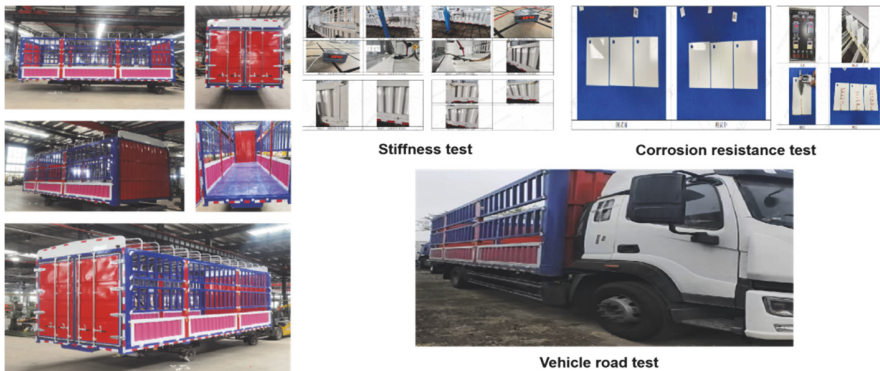
Fig. 9. hot stamped cargo box and related performance testing
