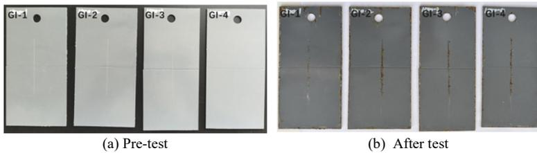
Fig. 5. Zinc based coated hot stamping steel.
