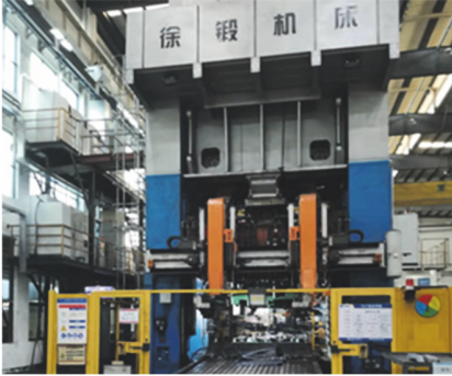
Fig. 1. Overall structure of the mechanical servo press
