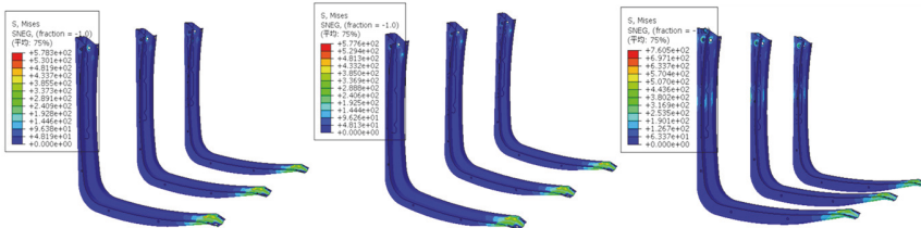
Fig. 5. Displacement cloud map of braking, steering, and impact conditions for hot forming scheme.
