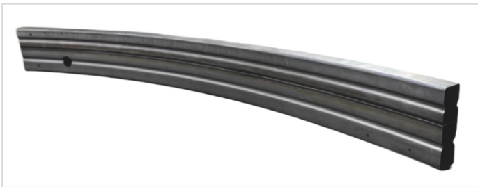
Fig. 12 Photographs of automobile bumper beams formed by roll forming and roll bending of high-strength steels
