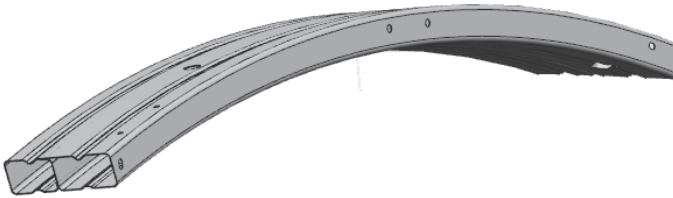
Fig. 7 Three-dimensional structure of the front bumper beam of a passenger car
