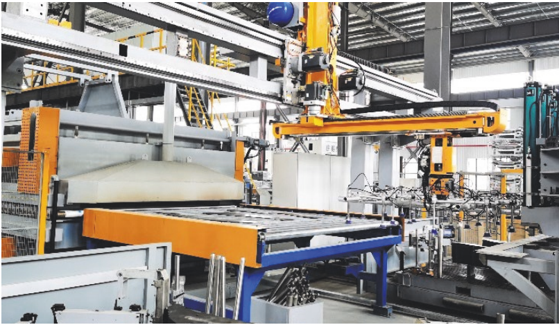
Fig. 7. Automatic transmission system for dismantling and heating furnace feeding
