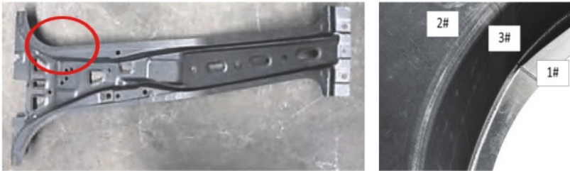
Fig. 6. Schematic diagram of tensile specimen taken from B-pillar.
