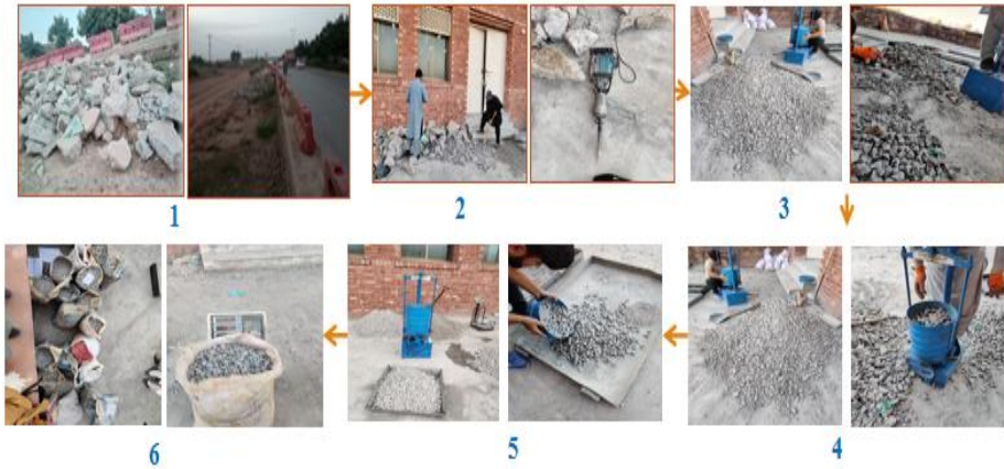
Fig. 4. Process involves extracting the required coarse aggregates
