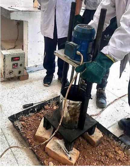
Figure 1: Mixing of agricultural waste in bitumen.
