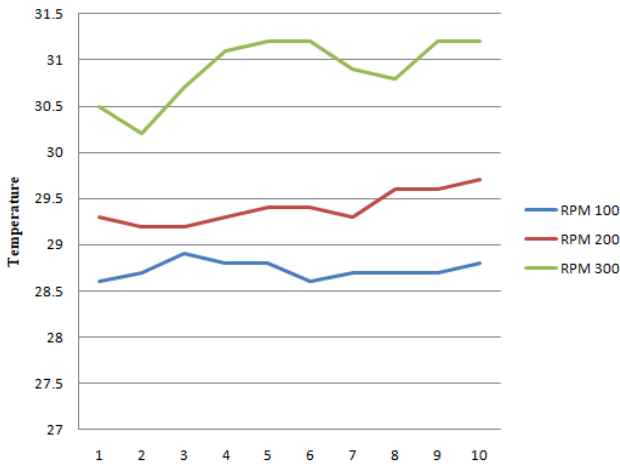
Figure 4. Material temperature after the grinding process
