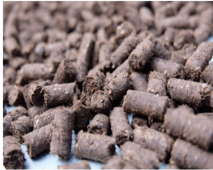
Figure 1. Solid waste is processed into pellets as fuel
