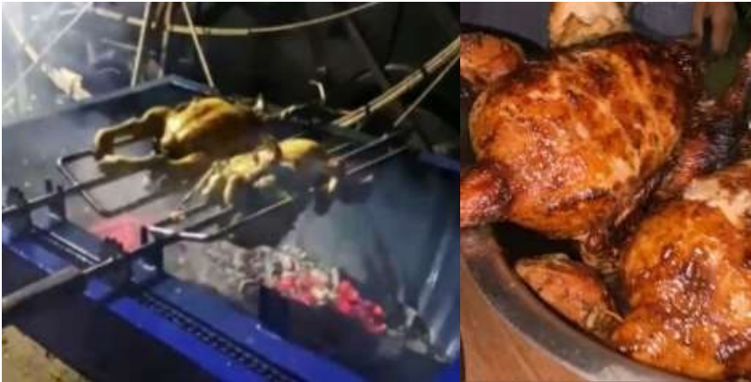
Figure 3. Test results showed 4 kg of chicken roasted for 60 minutes at 60°C, yielding evenly cooked and fully ripened meat
