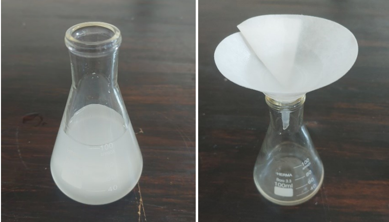
Figure 3. Lead solution used in adsorption tests (left) and filtration process: After shaking, the mixture is filtered using filter paper to separate solid hydroxyapatite from the solution (right)
