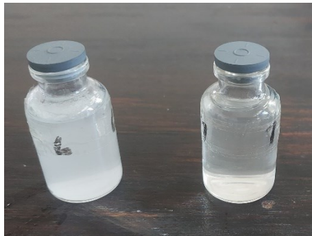
Figure 4. Solution comparison: Before filtration and after filtration with previously added hydroxyapatite adsorbent in vials
