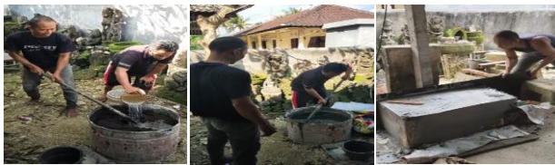
Figure 2. Molding process of artificial padas stone
